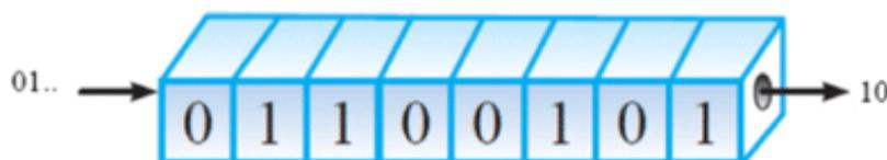
*Figure 6.4 bit transferring in SISO register*
