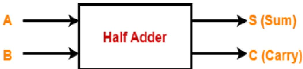
*Figure 3.7 Block Diagram of an half adder*
